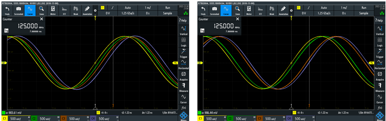
Figure 2.4: Phase aligned output generated by the above example showing channel 0 of slots 0, 1, 2 and 3 (left) as well as slots 0, 1, 4, 5 (right).
